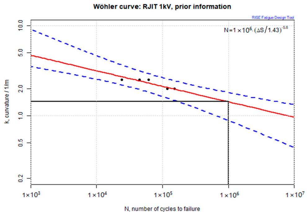
**Figure 7.** Estimated Wöhler curve of the cable, using prior knowledge on the exponent  $m$ , where the circles are experimental data, the solid line is the estimated Wöhler curve, and the dashed lines the 95% confidence intervals.
