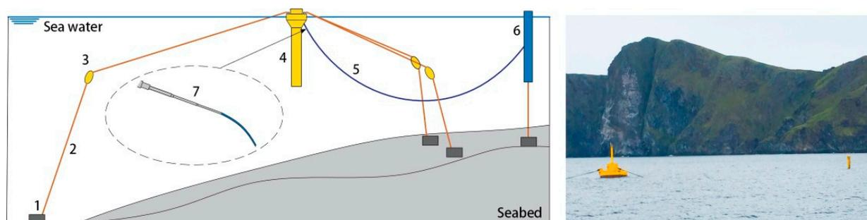
**Figure 1.** (Left) Illustration of the WaveEL 3.0 installation in Runde: (1) gravity anchor, (2) segment of a mooring line, (3) floater, (4) WEC, (5) cable, (6) hub, (7) bending restrictor, and (right) the full-scale WaveEL 3.0 system (photograph taken by the fourth author).
