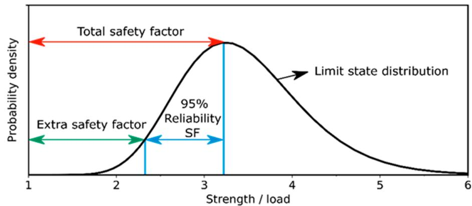
Figure 8. Load–strength limit state function.
